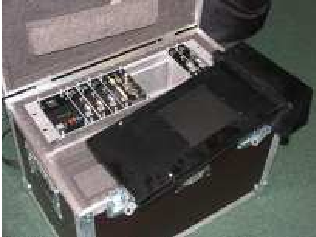
Figure 4. The “Bonn” shutter system for the 10k camera. This custom made shutter (black device) comes with control electronics to fit into a standard rack.
